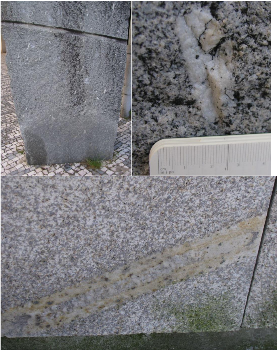
Figure 2. Examples of features of geological interest (FGIs) in built environment: biotitic porphyritic granite (upper left hand); twinning on feldspar (upper right hand); aplite-pegmatite textures in a veinlet of a two-mica granite (lower image).
